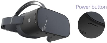
Start the VR headset by pressing the power button for 3 seconds. This button is located on the bottom of the VR headset on the right side.
